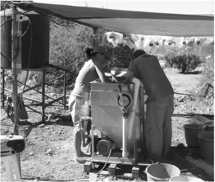
Figure 10. Flote-Tech machine-assisted flotation device in use at Mycenae. Photo courtesy of Brooke Hundtoft.
