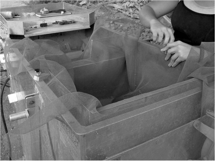
Figure 6. Student clipping cloth mesh to the interior of the main tank.
