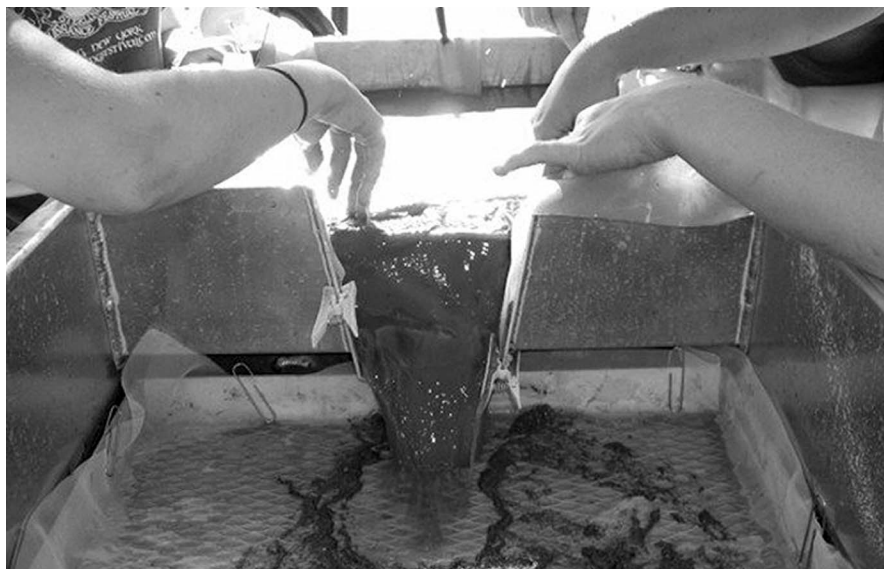
Figure 8. Photograph showing the flow of water from the main tank over the sluiceway and into the flot mesh.
