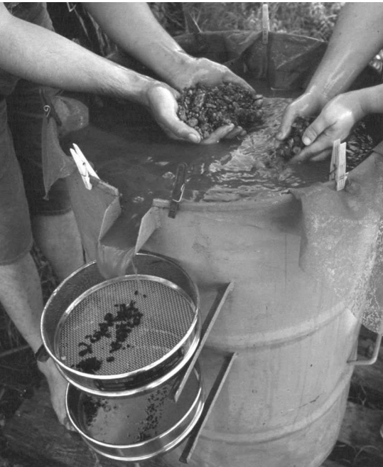
Figure 1. A water separation machine in use at Platamonas in northern Greece. The main tank has been modified from an oil drum by cutting the rim to accommodate the sluiceway. Photo courtesy of Evi Margaritis.
