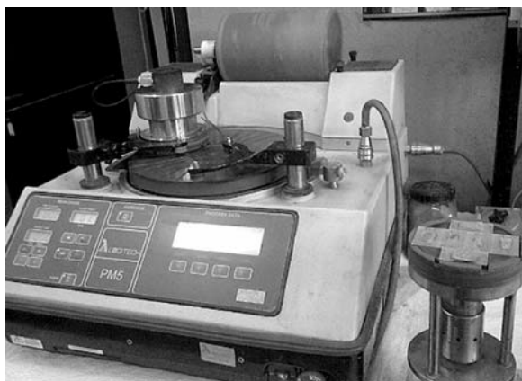
Figure 4. Lapping machine used to grind thin sections to a desired thickness. Photo by Eleanor Huffman.
